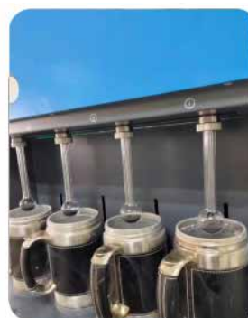
520ml stainless steel Dewar plated with cooper which can buff liquid nitrogen volatilization. Can be used at least 5 years.
